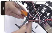
将接收机放进机身并用双面贴粘好 Put the receiver into the body and stickup with double paste.
