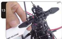
将主旋翼固定好 Fix up the main blade.
