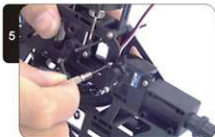
将左右副翼舵机固定 Fix the left and right AILE servos.
