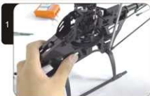
把脚架安装在机身上 Assembly the landing skid onto the body.
