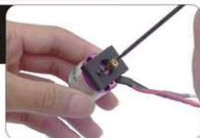
用螺丝把马达和固定座拧紧 Fix up the motor and mount with screws.
