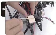
将调速器用双面贴粘好并固定 Stickup the ESC with double paste and fix it.
