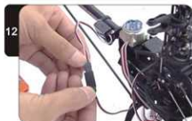
将陀螺仪和方向舵机连接 Connect the gyro and rudder servo.
