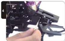
将前后升降舵机固定 Fix the front and rear ELEV servos.
