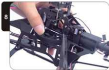
用球头钳把拉杆连上 Connect the push-rod with the bulb clipper.
