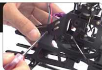
再把马达固定在机身上 Fix the motor on the body.
