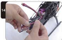
将调速器和马达连接 Connect the ESC and motor.
